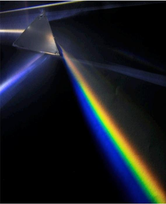
Fig. 3.3 Triangular prism dispersing light (normal dispersion).
