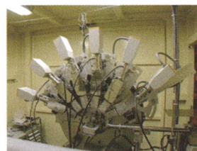
Synchrotron powder diffractometer with multiple-detection systems.
