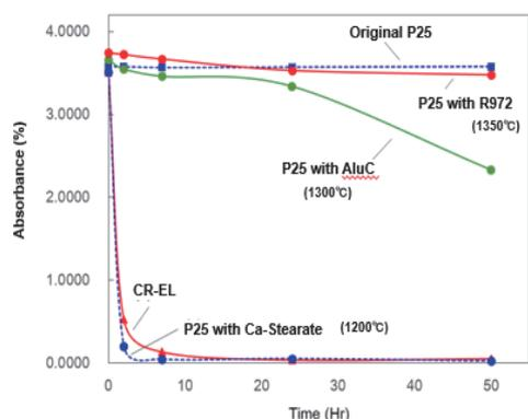
**Fig. 8** Sedimentation results of  $\text{TiO}_2$  dispersion
