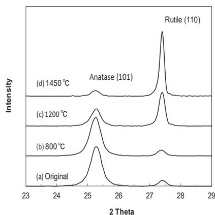
Fig. 2 XRD patterns of thermally-treated P25
