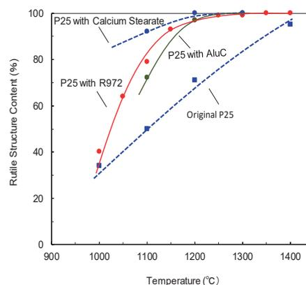
Fig. 7 Rutile conversion ratio for thermally-treated P25 mixed with external additive
