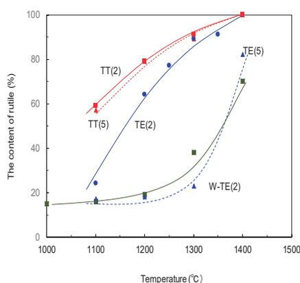
Fig. 5 Rutile conversion rate for thermally-treated P25
