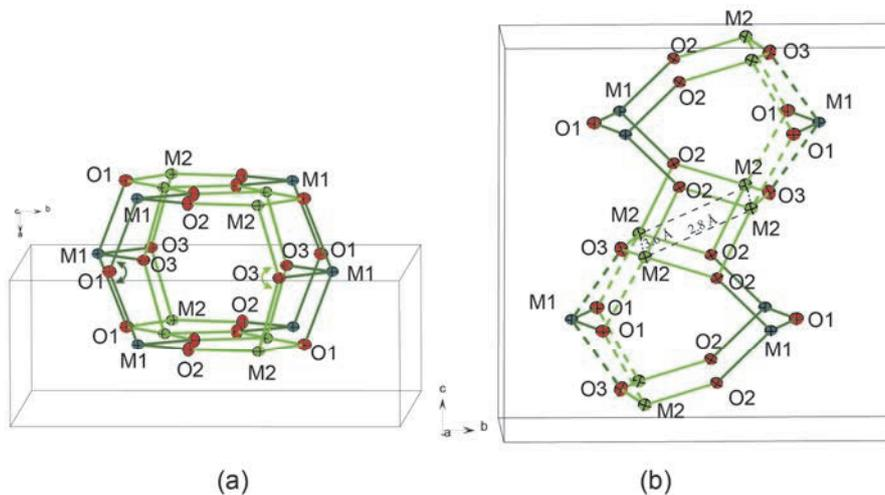
**Figure 11.** A structural tunnel running in the pseudobrookite-type  $\text{M}_1\text{M}_2\text{O}_5$  structure, viewed along a direction close to (a) the  $c$ -axis and (b) the  $a$ -axis. The chevron angles about O1 in the M1–O1–M1 pillar and that about O3 in the M2–O3–M2 pillar are shown by round arrows in (a).
