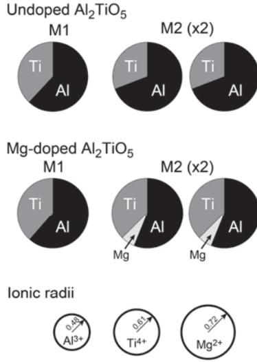
**Figure 2.** Distribution of metal atoms at the M1 (4c) and M2 (8f) sites in the undoped  $\text{Al}_2\text{TiO}_5$  at 322 K and Mg-doped  $\text{Al}_2\text{TiO}_5$  at RT. Two pie charts are drawn for M2 in accord with the ratio in number of the M1 and M2 sites. The ionic radii of  $\text{Al}^{3+}$ ,  $\text{Ti}^{4+}$  and  $\text{Mg}^{2+}$  in six-fold coordination with oxygens are shown at the bottom.
