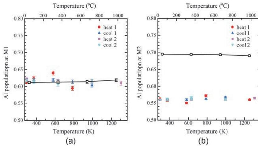
**Figure 3.** Aluminum population at (a) M1 and (b) M2 sites in the pseudobrookite-type  $^{[4c]}M1_1^{[8f]}M2_2O_5$  structure. The open circles connected by black polyline are data obtained from the undoped  $\text{Al}_2\text{TiO}_5$  during heating. The other scattered marks are those obtained from the Mg-doped  $\text{Al}_2\text{TiO}_5$  during the first heating/cooling and the second heating/cooling processes. The relationship between the colour marks and processes is shown in the legend.
