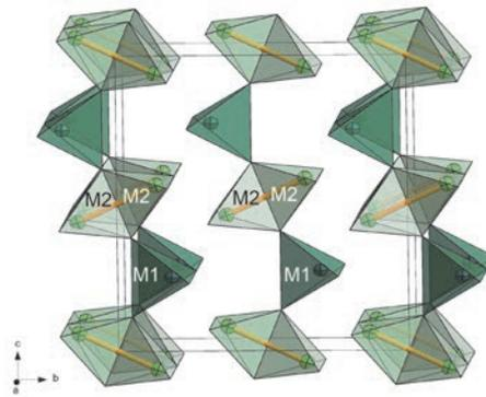
**Figure 8.** Tetrahedral drawing of the pseudobrookite-type structure, neglecting two long M–O bonds (dashed lines in **Fig. 6**) from the  $MO_6$  octahedra. The very short M2–M2 interatomic distance of  $\sim 2.8$  Å between the edge-sharing  $M_2O_4$  tetrahedra is shown by the yellow line.
