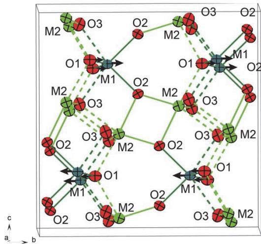
**Figure 6.** The room-temperature structure of the pseudobrookite-type  $M_1M_2O_5$  ( $Al_2TiO_5$ ), projected along a direction close to the  $a$ -axis. The thermal ellipsoids are drawn at 90% probability level. The shorter ( $\leq 2$  Å) and longer ( $> 2$  Å) M–O bonds are drawn by solid and dashed lines, respectively. The arrows attached to M1 and O1 indicate the direction of displacements of these atoms during heating.
