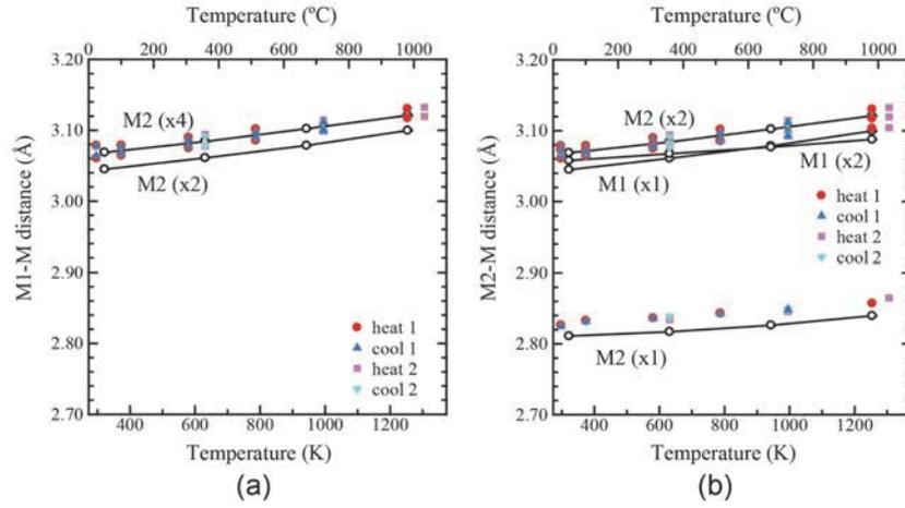
**Figure 10.** Temperature changes in the six M–M distances from the shortest around (a) M1 and (b) M2. The open circles connected by polyline are data obtained from the undoped  $\text{Al}_2\text{TiO}_5$  during heating. The other scattered marks are those obtained from the Mg-doped  $\text{Al}_2\text{TiO}_5$  during the first heating/cooling and the second heating/cooling processes. The relationship between the colour marks and processes is shown in the legend.
