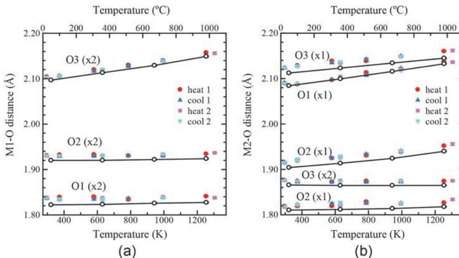
**Figure 7.** Temperature changes in the (a) M1–O and (b) the M2–O interatomic distances. The open circles connected by polyline are data obtained from the undoped  $Al_2TiO_5$  during heating. The other scattered marks are those obtained from the Mg-doped  $Al_2TiO_5$  during the first heating/cooling and the second heating/cooling processes. The relationship between the colour marks and processes is shown in the legend.
