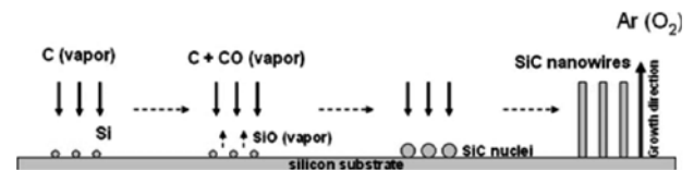
Fig.4 Schematic illustration of the SiC nanowires growth via VS mechanism [40] .
