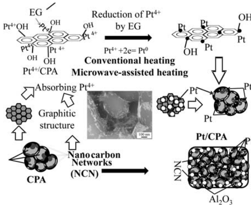
Fig. 6. Schematic of Pt nanoparticles deposition via different heating methods (EG: Ethylene glycol)
