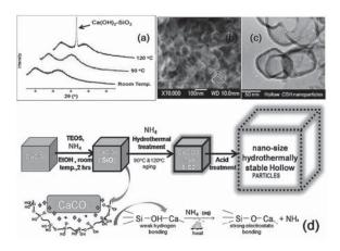
**Fig. 6** General Illustration of stabilization and formation of hollow calcium silicate hydrate particles by ammonia-hydrothermal template process.<sup>64</sup>
