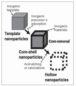
**Fig. 2** General schematic illustration of anisotropic HP using inorganic template approach.
