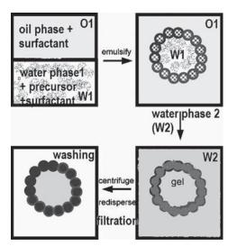
**Fig. 4** Basic illustration of double emulsion method (W<sub>1</sub>OW<sub>2</sub>)
