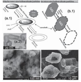
**Fig. 3** Schematic illustration and typical images of the anisotropic template process to form NMHSP <sup>36), 37)</sup> using colloidal nano-size CaHAp (a.1, a.2, a.3) and micro-size CaCO<sub>3</sub> particles (b.1, b.2)
