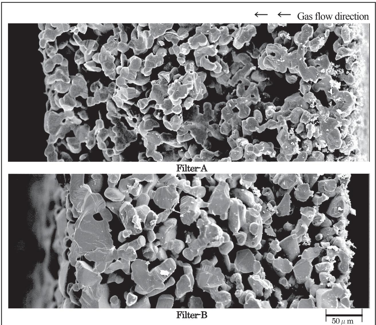
Fig. 12 SEM image of wall cross section
