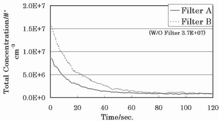
Fig. 8 Total concentration of particle which leaked from the outlet side of DPF in the initial 2 minutes.
