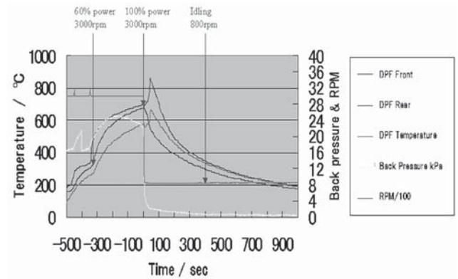
Fig. 5 Drop to idle test
