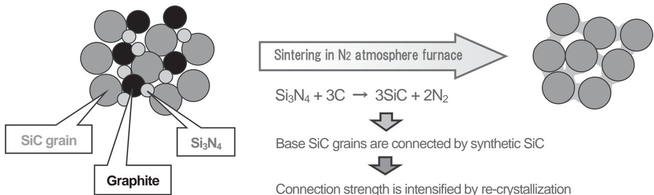
Therefore, since this sintering process is completed in shorter time and lower temperature as compared with the usual high temperature sintering, abnormal grain growth is restricted. Moreover, the control of porosity and pore size is easy, and lead to energy saving by this sintering process. The sintered filter element body shows a characteristic dark green color.
