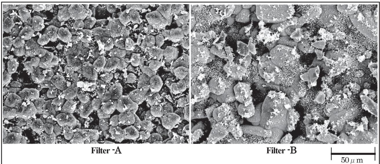
Fig. 11 SEM image of wall surface
