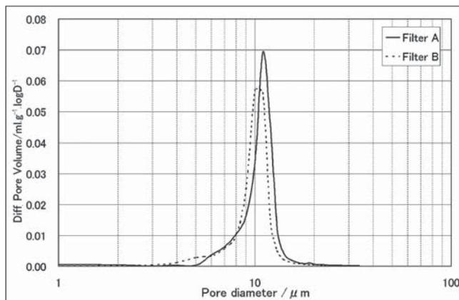
**Fig. 2** Pore size distribution of DPF test sample.
