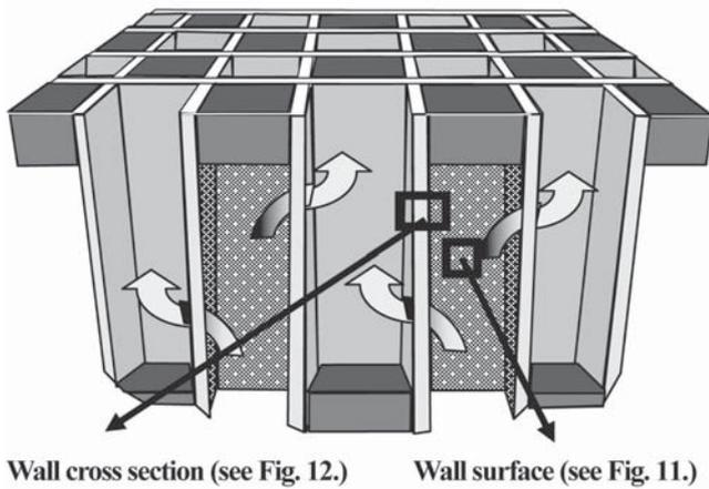
Fig. 13 SEM observation parts in the test samples.
