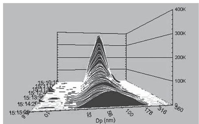
Fig. 10 Particle concentration and size distribution (Filter-B)
