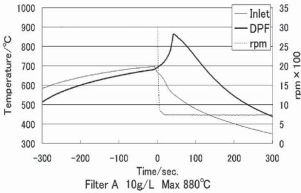
Fig. 6 DTIT Chart of Filter-A
