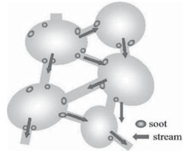
Fig. 14 Concept of microstructure in the wall.
