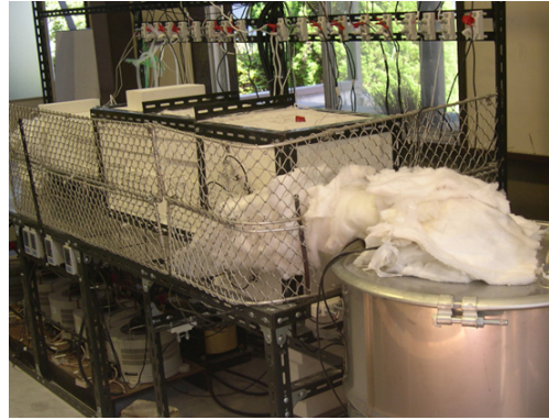
Fig. 3. View of the system 1 with a horizontal-type reaction chamber and exhaust gas processor.
