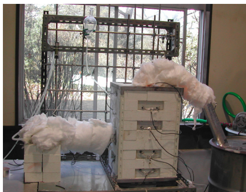
Fig. 5. View of the system 2 with a vertical-type reaction chamber in operation.
