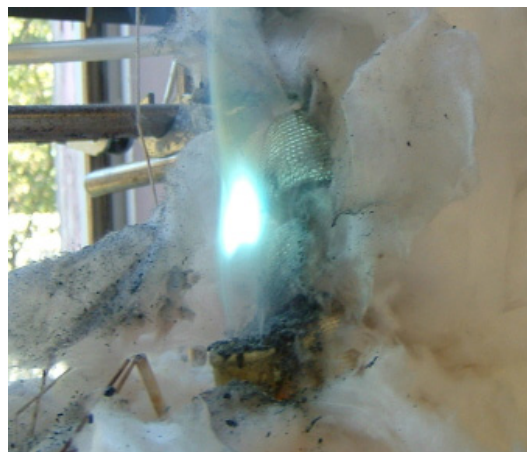
Fig. 4. Combustion of Zn gas at the top of exhaust pipe occurring when the \text{Al}_2\text{O}_3 extension tube is removed.
