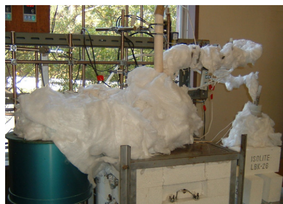
Fig. 2. View of the system. Zn gas is supplied from the left and \text{SiCl}_4 from the right to the reactor in the centre with an \text{Al}_2\text{O}_3 exhaust pipe on the top.
