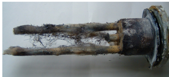
Fig. 6. Inside of reactor after the 1200 °C experiment.
