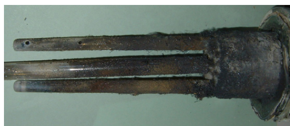
Fig. 7. Inside of reactor with short (top) and long (bottom) exhaust pipes after the 1250 °C experiment.
