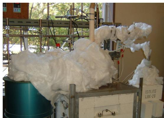
Fig. 2. View of the system. Zn gas is supplied from the left and  $\text{SiCl}_4$  from the right to the reactor in the centre with an  $\text{Al}_2\text{O}_3$  exhaust pipe on the top.
