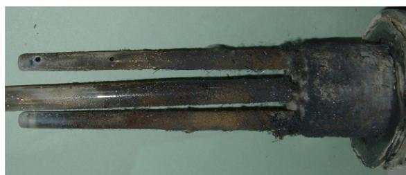
Fig. 8. Inside of reactor after the 1350 °C experiment.
