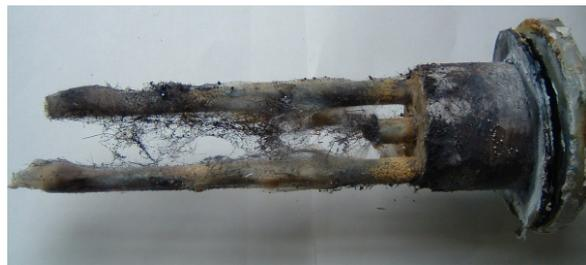
Fig. 6. Inside of reactor after the 1200 °C experiment.
