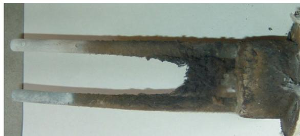
Fig. 7. Inside of reactor with short (top) and long (bottom) exhaust pipes after the 1250 °C experiment.
