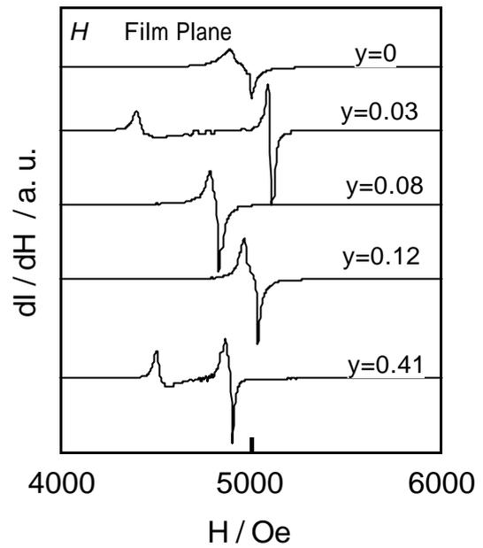
Fig.2. Ferromagnetic resonance spectra of the  $Y_{3-x}Gd_xFe_{5-y}In_yO_{12}$  at X band (9 GHz) region in the magnetic field perpendicular to the film plane. The measurements were performed at room temperature.
