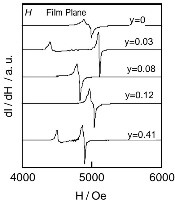
Fig.4. Ferromagnetic resonance spectra of the  $Y_{3-x-y}Gd_xCa_yFe_{5-y}Ti_yO_{12}$  at X band (9 GHz) region in the magnetic field perpendicular to the film plane. The measurements were performed at room temperature.
