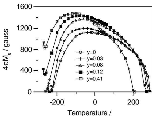
Fig.3. Temperature dependence of the saturation magnetization  $4\pi M_s$  of the  $Y_{3-x-y}Gd_xCa_yFe_{5-y}Ti_yO_{12}$  films.
