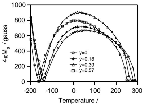
Fig.1 Temperature dependence of the saturation magnetization  $4\pi M_s$  of the  $Y_{3-x}Gd_xFe_{5-y}In_yO_{12}$  films
