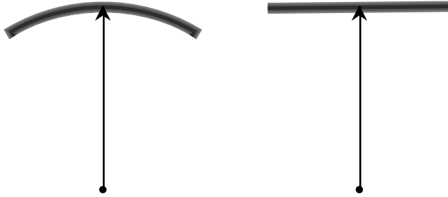
Fig. 6.6 The spherical plane for the diffraction condition (left) is approximated by a flat plane (right).
